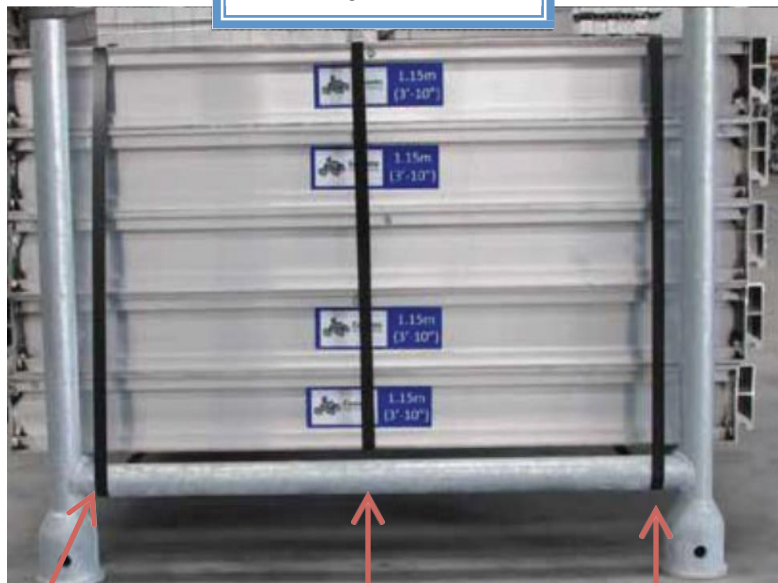
Band Beams & Barella at each end
