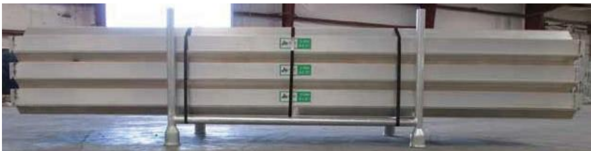
Main Beams must be nested. This is done by alternating the beams "right-side up" and then "up-side down"
