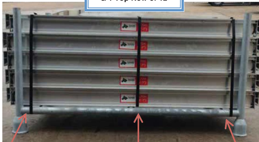
Band Beams & Barella at each end
