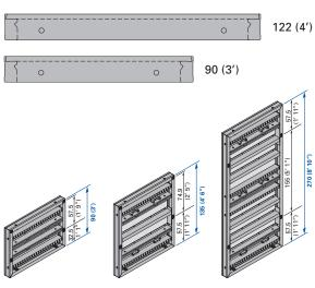
Framax Xlife universal panels are available in widths of 3'-0" (90 cm) and 4'-0" (122 cm) and in panel heights of 3'-0" (90 cm), 4'-6" (135 cm), 8'-10" (270 cm).
