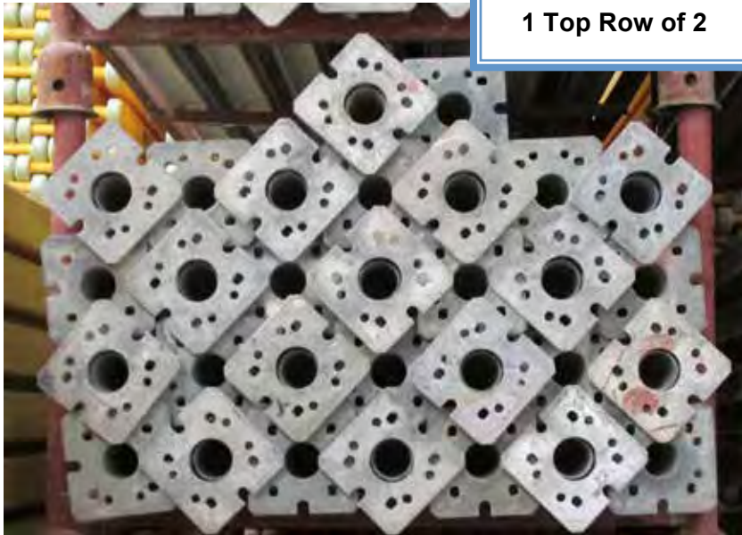
DO NOT leave Dropheads installed onto any HV Props or you will be subject to incur additional labor fees.
