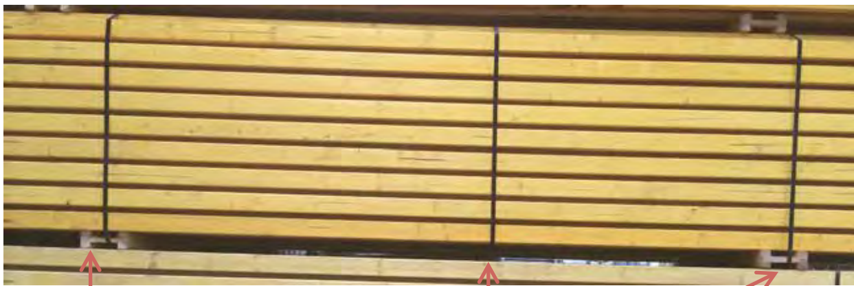
Band Dunnage with Girder on ends
